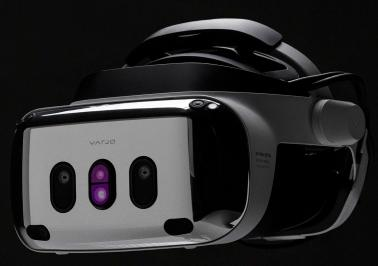
Dual 20-megapixel front mounted cameras and autofocus system improve near and far field vision and create the industry's best mixed reality experience.
